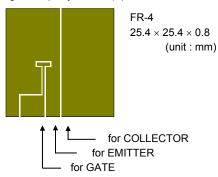
Note 2b : Device mounted on a glass-epoxy board (b)
